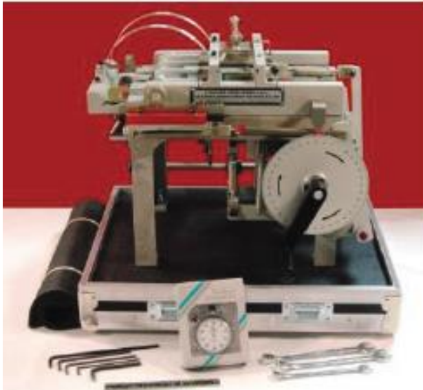
The Standard Timing Model (STM) is a mechanical skills assessment tool used to identify mechanical aptitude, skills, and instincts.
