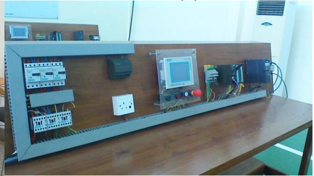
Several of the training stations are equipped with Siemens PLC and HMI equipment
